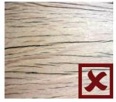
**Checking** is acceptable provided individual length does not exceed 250mm and width does not exceed 2mm.
