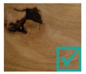
**Tight Knots** of less than 40mm in width are acceptable.
