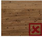
**Borer Holes** are acceptable provided there are less than 24 holes per 900mm depending on width.
